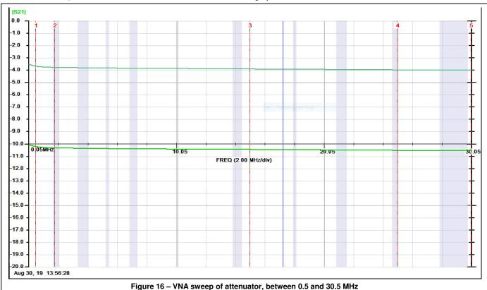
Figure 16 portrays a sweep using a VNA which shows the attenuation with, and without, the attenuator turned on. With the attenuator turned off (through the 22 and 270 ohm network) loss is about 4dB and with the attenuator turned on, it is slightly over 10dB.
