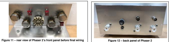
On the back panel, I added BNC connectors that are connected in parallel with the SO-239 UHF connectors, so there will never be a need for an adaptor (Figures 12 and 13).
