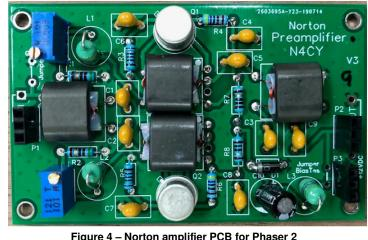
Figure 4 – Norton amplifier PCB for Phaser 2
