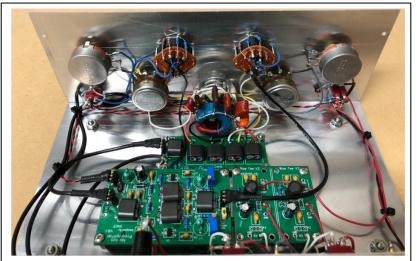
Figure 24 – Phaser #3 interior wiring
