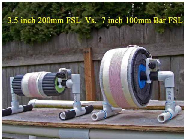
3) 3.5" Long-rod model (200mm ferrite length) deadlocks in weak-signal performance with 7" Bar model (100mm ferrite) **(7" Bar model FSL reception for the first 18 seconds, followed by that of the 3.5" Long-rod FSL)**
