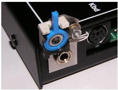
The NUE-PSK doesn't have a built in paddle, so I added a single lever paddle to it and it is just as easy to hike around and send CW with it as it is using a KX1. The paddle is made of an ALPS SSCF210300 Two Way Detector switch which is mounted on the side of the NUE-PSK case. It is useable up to 20 wpm. The NUE-PSK is just a little bit bigger than an Elecraft KX1.
