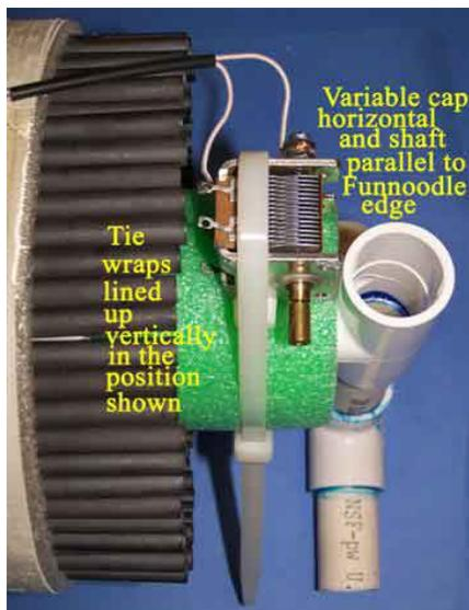
29) After the variable cap is secured tightly against the Funnoodle
