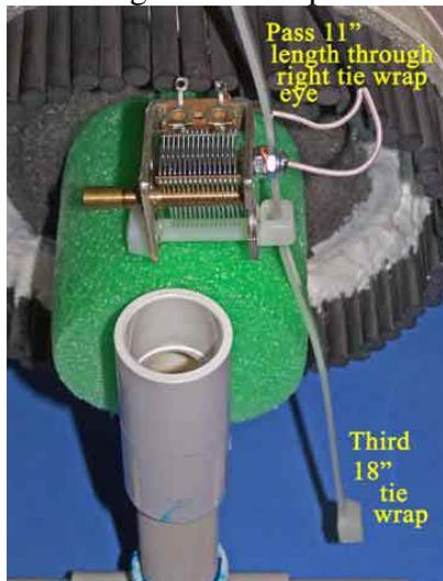
Litz wires and over the top of the variable cap, as shown.
