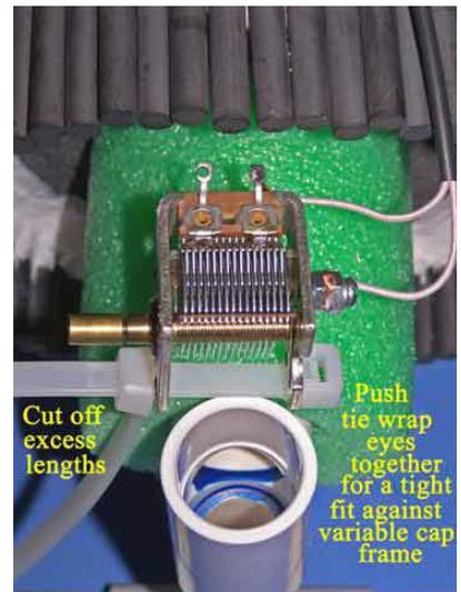
27) Refer to the photo below for the following step. Take the remaining 18" tie wrap and insert its end up through the right side tie wrap eye (as shown in the photo) for a length of 11", passing the tip in between the
