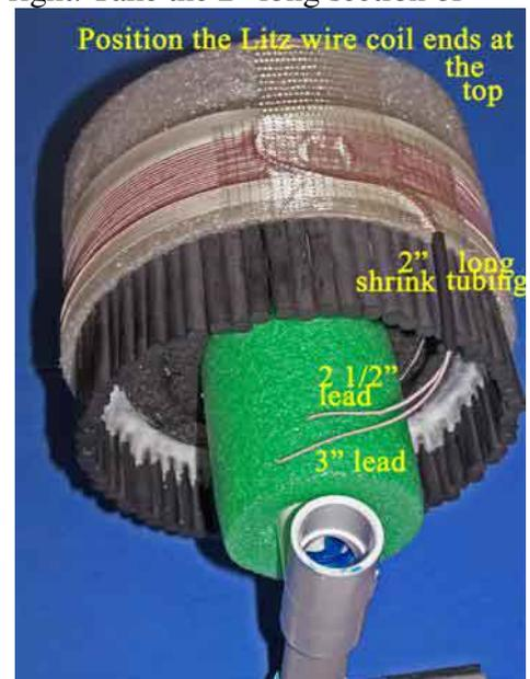
Scotch "Extreme" tape surface. In this position, the shrink tubing will protect the Litz wires from the sharp edges of the ferrite rods (in the sleeve assembly) during future operation.
