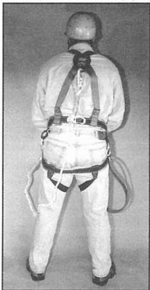
Photo 2: Rear view of climber. The fall arrest lanyard is connected to the D-ring between the shoulder blades.
