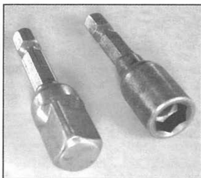
Photo 4: Drill socket driver for 3/8" sockets and 5/16" nut setter for hose clamps.
