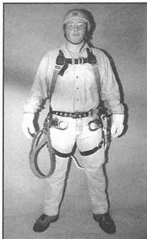
Photo 1: The well-dressed climber. Note the positioning lanyard on the left waist D-ring and the end of the fall arrest lanyard on the right D-ring.
