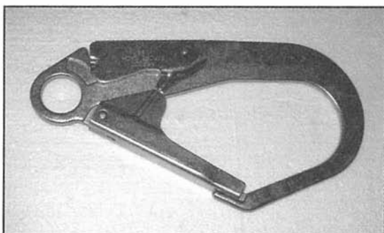
Photo 3: A rebar or gorilla hook. The mouth will open 2.5".
