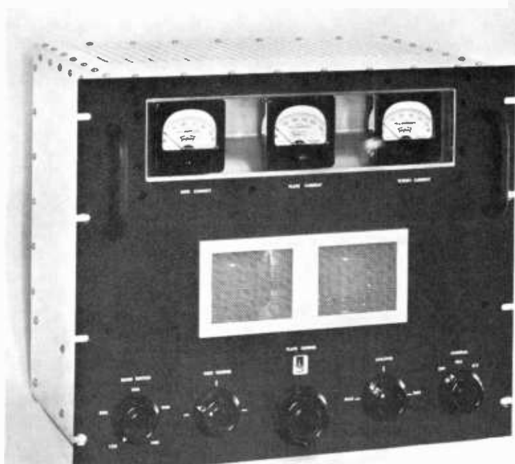
Figure 45 GENERAL PURPOSE AMPLIFIER OPERATES IN CLASS A, B, OR C MODE
