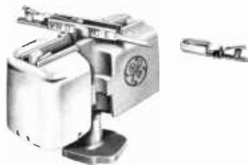
Figure 8 "RELUCTANCE" CARTRIDGE IS STANDARD PICK-UP FOR MUSIC SYSTEM. Low stylus pressure of four grams insures minimum record wear. Dual stylus is used having two needle tip diameters for long playing and 78 R.P.M. recordings.
