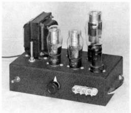
Figure 35. Regulated bias supply may be built upon small steel chassis. "Adjust bias" control is on front apron, and current adjustment potentiometer for regulator is next to power transformer.
