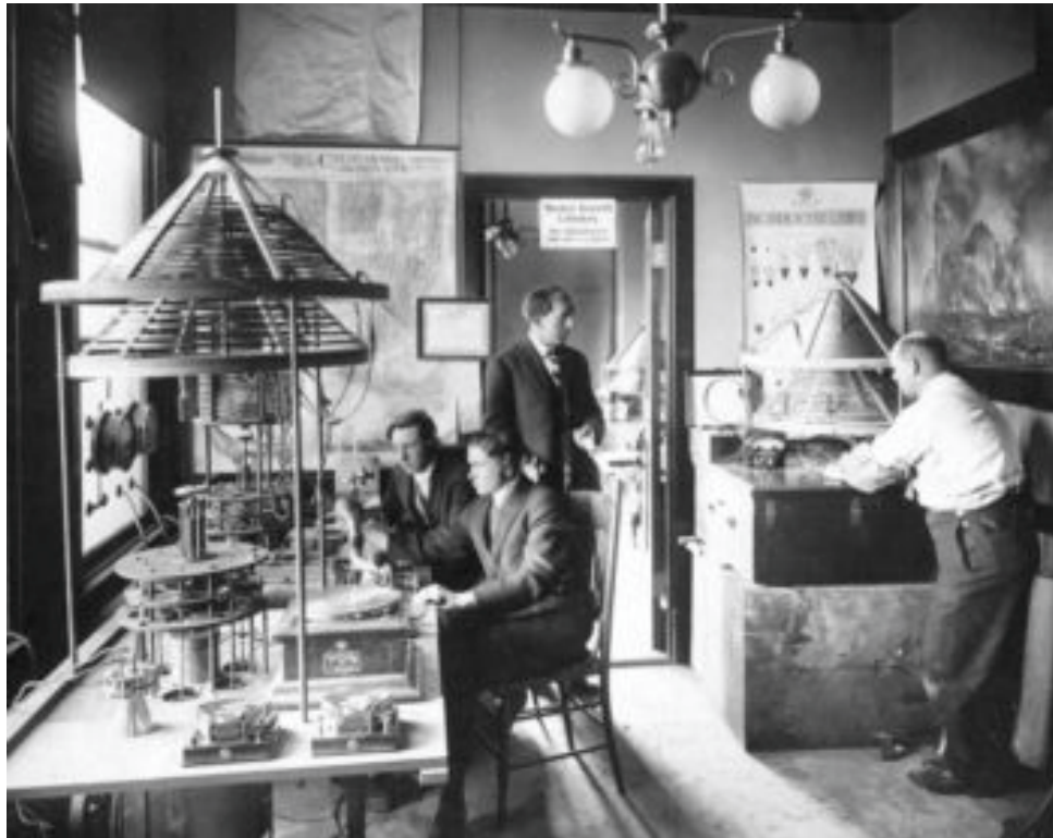
Charles "Doc" Herrold (standing, center) at his San Jose, Calif., combination radio school and broadcast station. The turntable (phonograph) and microphone (telephone carbon "transmitter") are clearly visible on the table at the left.
