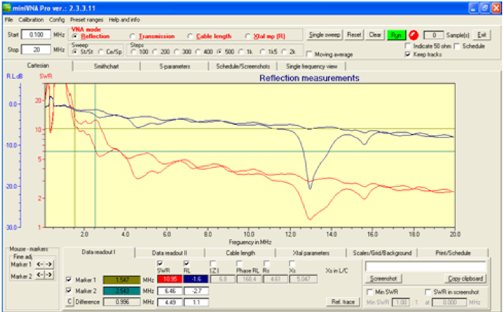
Figure 4: As in Figure 3 but for frequency range 0.1 to 20MHz and showing effect of reversing the coax connection to the copper loop.
