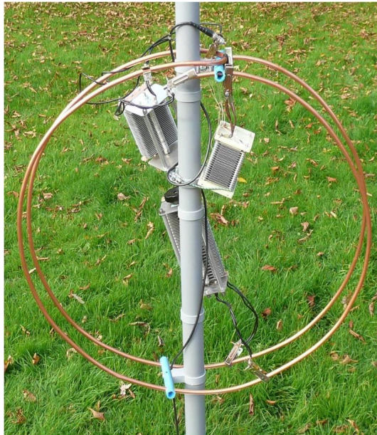
Figure 4 from [4]: 80cm two opposing turns double tuned coupled multi-mode loop transmit antenna 1.8 to 70MHz. Top-fed on left, and bottom fed schematic on right
