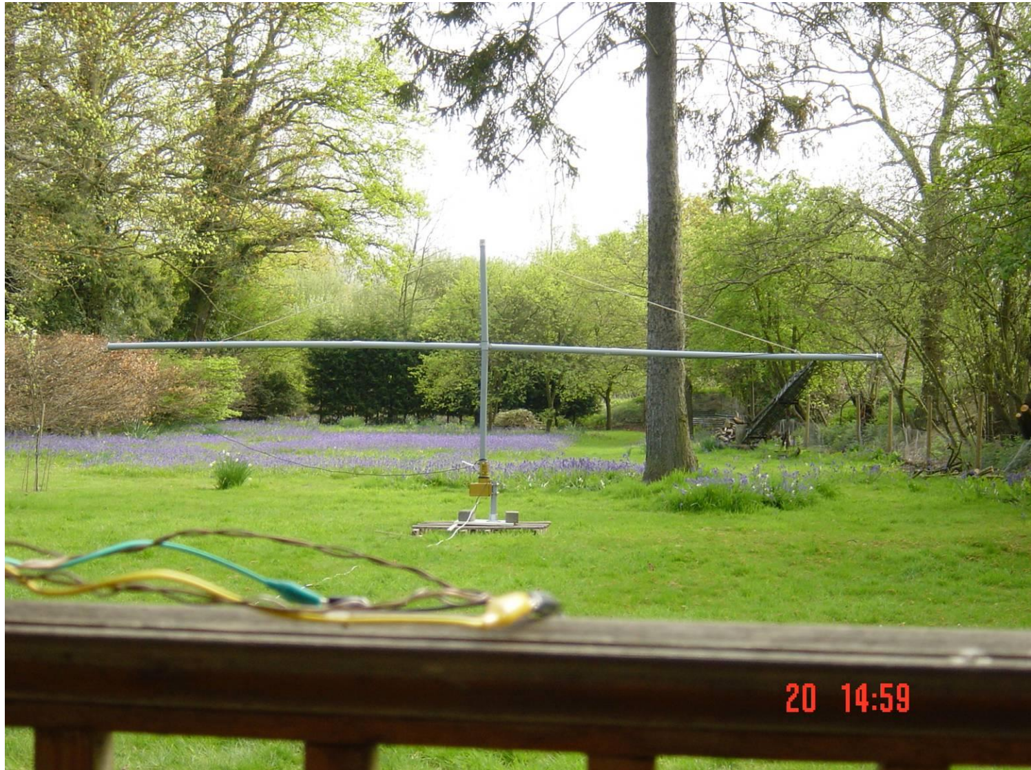
Figure 2: Underhill Research Open Range for Small Antenna Measurement. (Illustrating Rotatable 6.1m End-fed Horizontal Wire (inside plastic pipe) at 16m Distance with UR 35cm Receiving Loop in Foreground.)
