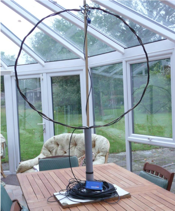
Figure 1 (on left): Picture of 90cm loop-monopole with MiniVNApro (Bluetooth connected) vector network analyser at bottom.
