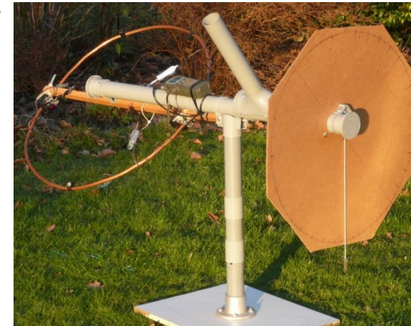
Figure 1: Tuned-Loop Goniometer with plumb-line reference and AOR8200 receiver. Tuning capacitors are on far left end of loop. Carefully balanced subsidiary segment shaped loop to receiver partially twisted around main loop conductor.
