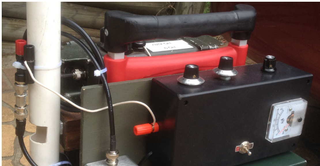
GTU mounted on trolley. Notice the wire connecting the coax antenna braid or screen to the GTU!
