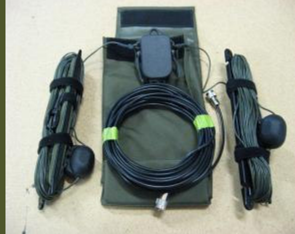
BU000185 Portable Tactical Broadband Dipole with braided Kevlar wire (3-30MHz)
