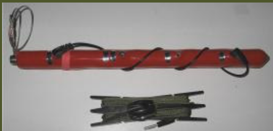
TJ-16 Firecracker Emergency antenna with Flexiweave wire.
