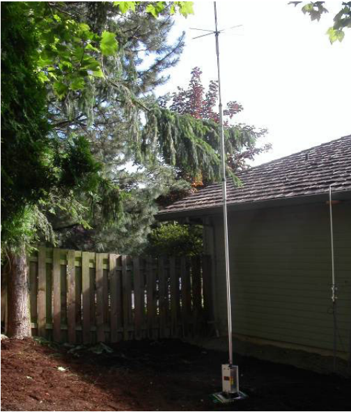
Ground-mounted multi-band antenna of a type standing 5.5 to 8 metres tall.
