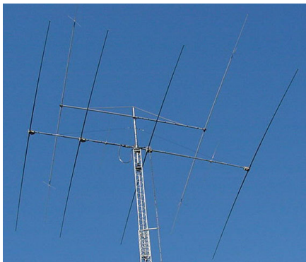
Telescopic metal-lattice mast with stacked rotatable HF Yagi beams.
