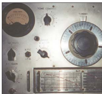
The restored RCA AR88D. This receiver is far from being in original condition, with its first RF stage replaced with an miniature EF183 valve and its metal cabinet replaced by a wooden one, made from Western Australian jarrah. However, it works well and is a great talking point.
