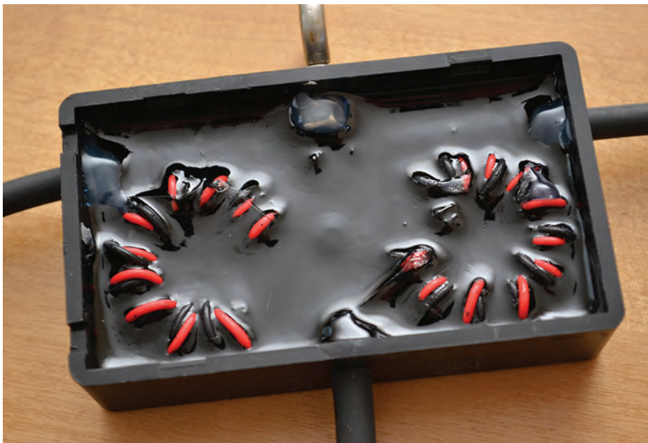
The balun uses two matched toroidal transformers potted in epoxy.
