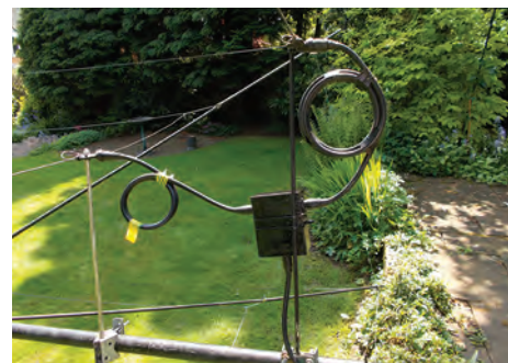
PHOTO 5: The diplexer attached to the 10m and 6m quads via quarter wave stubs. The connections were liberally waterproofed with self-amalgamating tape.
