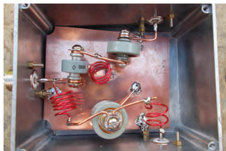
PHOTO 4: The completed diplexer. Input on the left, high pass output at the top of the photo and low pass at the bottom. Note the solder tags that connect the copper board to the bolts that secure the three SO-239 sockets.
