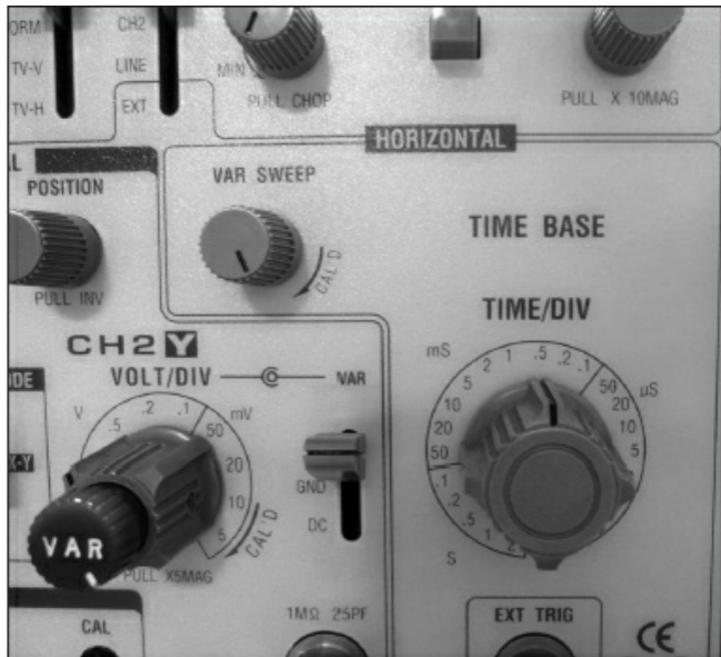
Figure 7.16 — The sweep rate or time base control is labeled here as TIME/DIV. Notice the variable control (VAR SWEEP) to its upper left.
