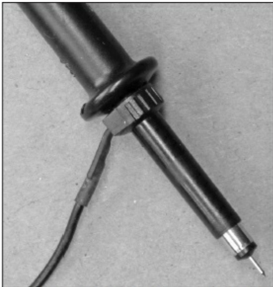
Figure 4.7 — When grabbing a component lead to be examined is not possible a pointed end is available to actually “probe” the circuit point.
