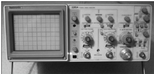
Figure 2.8 — The vacuum tube lab scopes were replaced by solid state lab scopes weighing perhaps one-fifth of the weight of their predecessors and requiring a tenth of the ac power. [Photo courtesy of Rich Roznoy, K10F]
