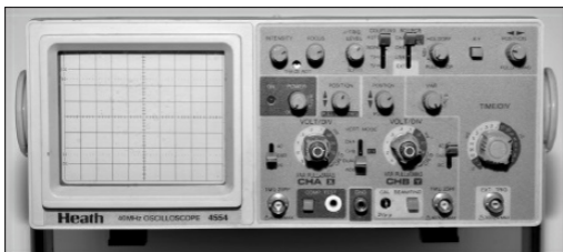
Figure 2.10 — Heath also upgraded from tubes to solid state and higher frequency performance. The input section of these kits looked more like a receiver front end than a piece of test equipment. [Photo courtesy of Seth Goltzer, W1SHG and Don Hudson, KA1TZR]
