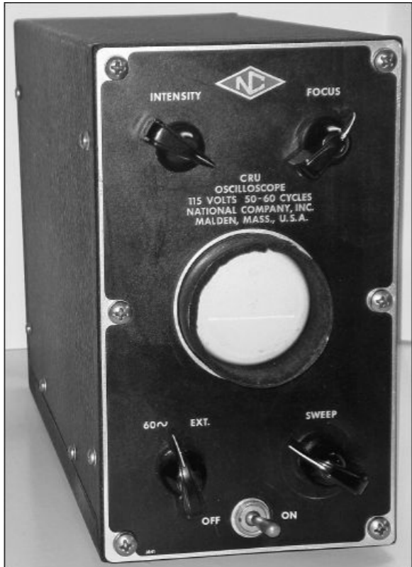
Figure 2.3 — After World War II, National came out with a new scope, featuring a larger tube. [Photo courtesy of Chuck at myvintagetv.com]
