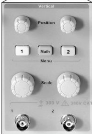
Figure 6.6 — A key button on this self-contained modern Tektronix oscilloscope is the one labeled MATH as shown in the closeup. It allows you to combine the input signal in a variety of ways, in addition to performing a number of mathematical operations and measurements on the signals.
