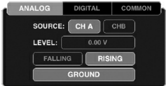
Figure A3.3 — The trigger selection menu has a variety of options. In this case analog channel A has been selected. Right now it show 0 V or ground has been selected, By taping on the LEVEL window a set of sliders appears that allows direct trigger voltage selection.
