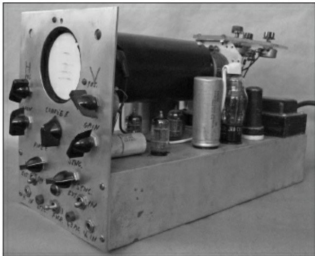
Figure 2.A — Tim Walker, W1GIG, built this oscilloscope as a clone of the Heath scope over 50 years ago. Notice the graticule (screen divisions) consists of markings made with a grease pencil!
