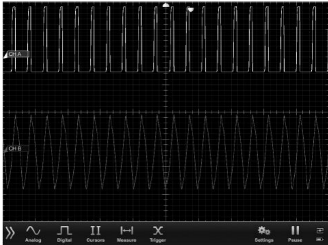
Figure A3.1 — Dual inputs at 100 kHz. The narrow rectangular pulses on channel A are not really synchronized with the triangular pulses on channel B. They only appear that way because the trigger selection was tweaked to make them line up.
