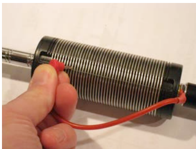
Figure 44 Quick tuning the Buddistick
