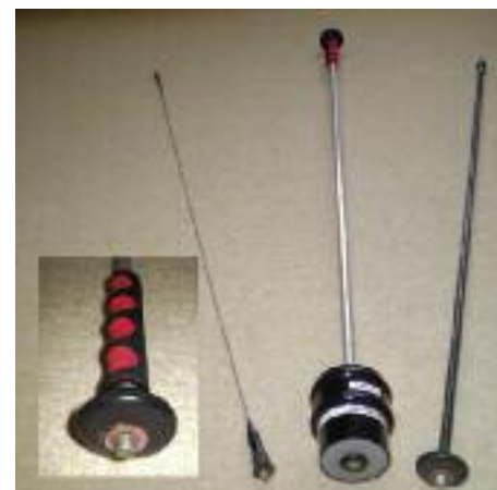
PHOTO 2: The centre-loaded 20m antenna is typical of my construction. Inset left: detail of the antenna mounting screw.
