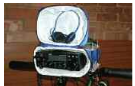
The Alinco DX-70 mounted in a weatherproof covering on the bike handlebars.
